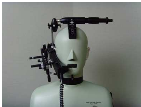
Figure 1: Client 1 Handset in HATS jig
