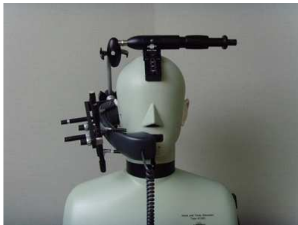
Figure 2: Client 2 Handset in HATS jig
